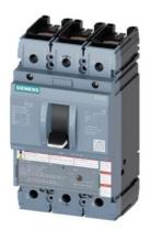
circuit breaker 3VA5 UL frame 250 breaking capacity class C 100kA @ 480 V 3-pole, line protection TM210, FTFM, In=50A overload protection Ir=50A fixed short-circuit protection Ii=10 x In cable connection on on both sides
