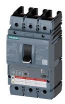
circuit breaker 3VA6 UL frame 250 breaking capacity class C 100kA @ 480V 3-pole, line protection ETU320, LI, In=250A overload protection Ir=100A...250A short-circuit protection li=1.5...10 x In without connection
