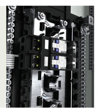
**Note:** Tandem AFCI breakers without the rejection feature can be installed in any panel that lists this specific breaker type or where a substitution letter exists for that breaker type. The schematic located on the wiring diagram will show the positions where these breakers can be placed by showing two circuits per space. The total circuits listed for panel should not be exceeded.
