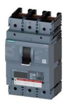
Circuit breaker 3VA6 UL Frame 600 breaking capacity class M 35kA @ 480V 3-pole, Line protection ETU820, LI, In=400A overload protection, 100% rated Ir=160A...400A Short-circuit protection Ii=1.5...12 x In without connection
