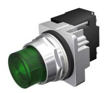
30mm Command/52, Chrome Finish Heavy Duty,Watertight/Oiltight Complete Metal Unit Illuminated Indicator Light Transformer type, 240V AC LED Lamp, BA9s Plastic Lens, Green UL Listed, CSA Certified NEMA 1,3,3R,4,4X,12,13 & Automotive Standards
