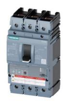
circuit breaker 3VA6 UL frame 250 breaking capacity class C 100kA @ 480 V 3-pole, line protection ETU320, LI, In=100A overload protection Ir=40A ...100A short-circuit protection Ii=1.5...12 x In cable connection on both sides
