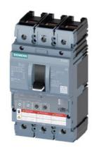
circuit breaker 3VA6 UL frame 250 breaking capacity class C 100kA @ 480 V 3-pole, line protection ETU350, LSI, In=250A overload protection Ir=100A ...250A short-circuit protection Isd=1.5... 10 x Ir, Ii=10 x In cable connection on both sides
