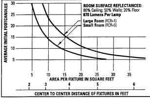
Use quick calculator chart to determine the spacing of 60 Watt A19 units for a desired level of illumination.
