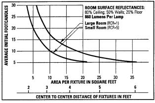
Use quick calculator chart to determine the spacing of 13 Watt Quad Tube units for a desired level of illumination.
