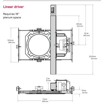
Dimensions for DALI 4800lm & 6000lm, & RA light engines.
