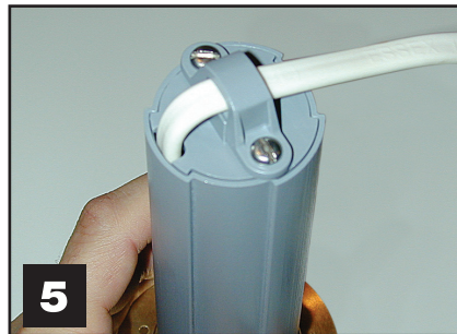
Figure 5 - Secure wire clamp on bottom of tube.
