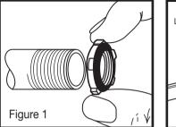
1. Thread sealing locknut onto conduit up to end of thread, as shown in Figure 1.
