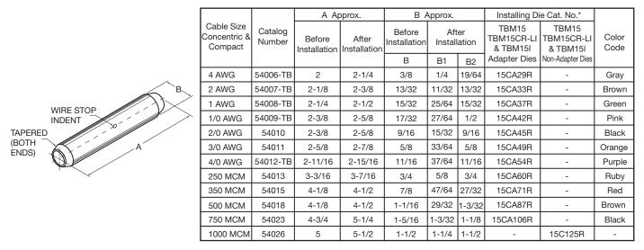
\*THESE DIES ARE RECOMMENDED FOR ALL HIGH VOLTAGE (UP TO 15KV) APPLICATIONS. THEY ARE DESIGNED TO YIELD A SMOOTH ROUND CONNECTOR WHEN CRIMPED ACCORDING TO THESE RECOMMENDATIONS ON THIS SHEET. THEY ARE DISTINGUISHED FROM THE EQUIVALENT HEX DIES BY THE SUFFIX "R".
