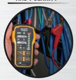
**MAP WIRES TO CHECK PIN-TO-PIN** CONNECTIONS
