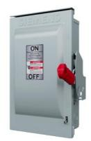
Siemens Low Voltage Circuit Protection Heavy Duty Safety Switch. 3-Pole Non-Fused in a type 3R enclosure (outdoor). Rated 600VAC (100A).
