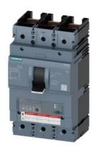
circuit breaker 3VA6 UL frame 400 breaking capacity class C 100kA @ 480V 3-pole, line protection ETU320, LI, In=400A overload protection Ir=160A...400A short-circuit protection Ii=1.5...10 x In without connection
