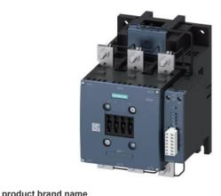
power contactor, AC-3e/AC-3 225 A, 110 kW / 400 V AC (50-60 Hz) / DC Uc: 96-127 V PLC input 24 V DC 3-pole, auxiliary contacts 1 NO + 1 NC drive: electronic main circuit: busbar control and auxiliary circuit: screw terminal with remaining lifetime indicator
