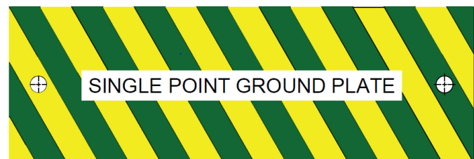
FAA3 = SINGLE POINT GROUND PLATE* Alternating Green and Yellow stripes
