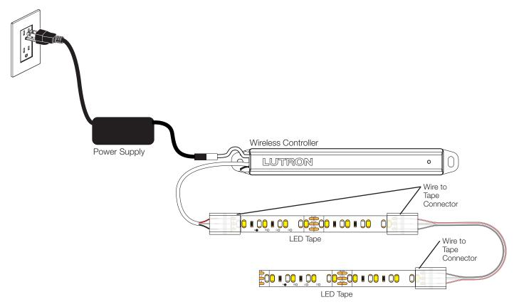
• The length of the 24 V== cable coming from the power supply may be extended by cutting the plug ends off both the power supply and the wireless controller and adding cable of the appropriate gauge, from the table below to account for the distance.
