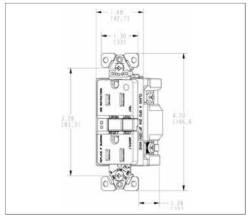
Figure 3. SGFH15 Line art with dimensions
