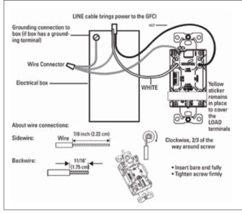
Figure 1. One cable (2 or 3 wires) entering the box
