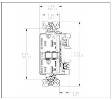
Figure 4. SGFH20 Line art with dimensions
