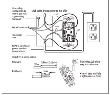
Figure 2. Two cables (4 or 6 wires) entering the box
