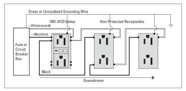
Figure 5. OBC AFCI: Feed-Through Installation with Non-Protected Receptacles Downstream
