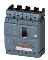
CIRCUIT BREAKER 3VA5 UL Frame 400 BREAKING CAPACITY CLASS M 35kA @ 480 V 4POLE, LINE PROTECTION TM230, FTAM, In=300A OVERLOAD PROTECTION IR=300A FIXED SHORT CIRCUIT PROTECTION Ii=5...10 x In NEUTRAL UNPROTECTED W/O CONNECTION
