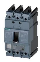
circuit breaker 3VA5 UL frame 125 breaking capacity class M 35kA @ 480 V 3-pole, line protection TM230, FTAM, In=90A overload protection Ir=90A fixed short-circuit protection Ii=5...10 x In without connection
