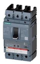
circuit breaker 3VA6 UL frame 150 breaking capacity class M 35kA @ 480V 3-pole, line protection ETU350, LSI, In=150A overload protection Ir=60A...150A short-circuit protection Isd=1.5...10 x Ir, Ii=10 x In without connection
