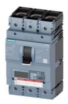
circuit breaker 3VA6 UL frame 400 breaking capacity class C 100kA @ 480 V 3-pole, line protection ETU556, LSI, In=400A overload protection Ir=160A ...400A short-circuit protection Isd=0.6..10x In, Ii=1.5..10x In N conductor protection opt. w. ext. CT; up to 160% ground-fault alarm message via EFB300 or COM cable connection on both sides
