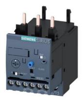
Overload relay 10...40 A Electronic For motor protection Size S0, Class 20 Contactor mounting Main circuit: Screw Auxiliary circuit: Screw Manual-Automatic-Reset
