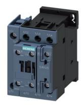
contactor AC-1, 40 A, 400 V / 40 °C, 4-pole, 24 V AC, 50/60 Hz, auxiliary contacts: 1 NO + 1 NC, screw terminal, size: S0
