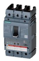
circuit breaker 3VA6 UL frame 150 breaking capacity class M 35kA @ 480V 3-pole, line protection ETU350, LSI, In=100A overload protection Ir=40A...100A short-circuit protection Isd=1.5...10 x Ir, Ii=12 x In without connection
