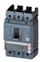
circuit breaker 3VA5 UL frame 250 breaking capacity class M 35kA @ 480 V 3-pole, line protection TM230, FTAM, In=100A overload protection Ir=100A fixed short-circuit protection Ii=5...10 x In without connection
