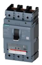
circuit breaker 3VA6 UL frame 400 breaking capacity class H 65kA @ 480V 3-pole, line protection ETU350, LSI, In=400A overload protection Ir=160A...400A short-circuit protection Isd=1.5...10 x Ir, Ii=10 x In without connection
