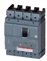
CIRCUIT BREAKER 3VA5 UL Frame 600 BREAKING CAPACITY CLASS M 35kA @ 480 V 4POLE, LINE PROTECTION TM230, FTAM, In=600A OVERLOAD PROTECTION IR=600A FIXED SHORT CIRCUIT PROTECTION II=4...8x In NEUTRAL UNPROTECTED W/O CONNECTION
