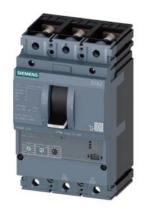
circuit breaker 3VA2 IEC frame 250 breaking capacity class C Icu=110kA @ 415V 3-pole, motor protection ETU350M, LSI, In=200A overload protection Ir=80A...200A short-circuit protection Isd=3...15 x Ir, Ii=15 x In nut keeper kit
