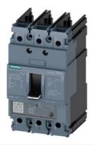
circuit breaker 3VA5 UL frame 125 breaking capacity class M 35kA @ 480 V 3-pole, line protection TM230, FTAM, In=60A overload protection Ir=60A fixed short-circuit protection Ii=5...10 x In without connection
