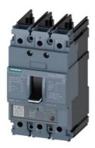
circuit breaker 3VA5 UL frame 125 breaking capacity class H 65kA @ 480V 3-pole, line protection TM230, FTAM, In=125A overload protection Ir=125A fixed short-circuit protection Ii=5...10 x In without connection
