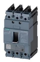
circuit breaker 3VA5 UL frame 125 3-pole, starter protection TM120M, AM, In=125A without overload protection short-circuit protection Ii=5...12 x In without connection
