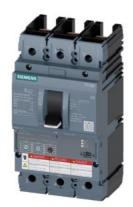
circuit breaker 3VA6 UL frame 150 breaking capacity class C 100kA @ 480V 3-pole, line protection ETU320, LI, In=100A overload protection Ir=40A...100A short-circuit protection Ii=1.5...12 x In without connection
