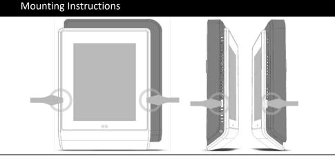
Using the appropriately sized tool, press in the release tabs of each sides of the device until to the backplate is noticeably released.
