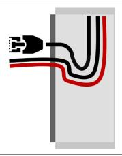
Pull all wires out of the wall and run them through central hole of the backplate. Screw the backplate onto the wall.
