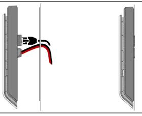
Plug the wire(s) into the connector(s), the gently push the excess wiring back into the wall. Reattach the front plate and ensure that it clips tightly to place. Tighten the security screw, if applicable.
