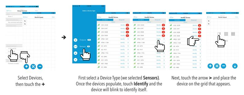
Note: To identify a switch, first press any button on the physical switch(s) to wake. Then touch device type **Switches**, and the list of awake switches will populate.
