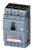
circuit breaker 3VA6 UL frame 400 breaking capacity class C 100kA @ 480 V 3-pole, line protection ETU350, LSI, In=400A overload protection Ir=160A ...400A short-circuit protection Isd=1.5... 10 x Ir, li=10 x In cable connection on both sides
