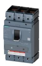
CIRCUIT BREAKER 3VA5 UL FRAME 400 BREAKING CAPACITY CLASS C 100kA @ 480 V 3POLE, LINE PROTECTION TM240, ATAM, In=400A OVERLOAD PROTECTION Ir=280A ...400A SHORT CIRCUIT PROTECTION Ii=5...10 x In NUT KEEPER KIT LINE AND LOAD S.
