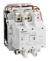
Mechanically held lighting contactor, Contactor amp rating 100A, 0 N.C. / 3 N.O. poles, 110VAC 50HZ/120VAC 60HZ coil, Non-combination type, Enclosure NEMA type (open), No enclosure
