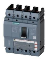
circuit breaker 3VA5 UL frame 250 breaking capacity class M 35kA @ 480V 4-pole, line protection TM210, FTFM, In=250A overload protection Ir=250A fixed short-circuit protection Ii=10 x In N conductor unprotected without connection
