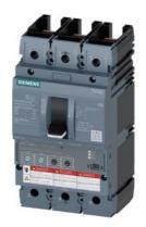
circuit breaker 3VA6 UL frame 150 breaking capacity class H 65kA @ 480V 3-pole, line protection ETU330, LIG, In=100A overload protection Ir=40A...100A short-circuit protection Ii=1.5...12 x In ground-fault protection Ig=0.2...1 x In, tg=0.1/0.3s without connection
