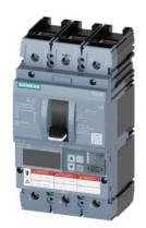
circuit breaker 3VA6 UL frame 150 breaking capacity class C 100kA @ 480 V 3-pole, line protection ETU560, LSIG, ln=150A overload protection Ir=60A ...150A short-circuit protection Isd=0.6..10x In, Ii=1.5..10x In N conductor protection opt. w. ext. CT; up to 160% ground-fault protection Ig=0.2... 1 x In, tg=0.05-0.8s cable connection on both sides
