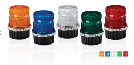
Model FB2LED is a multi-pattern LED available in single color and quad-color models. Single color models are available in five colors (Amber, Blue, Clear, Green, and Red) and feature Federal Signal's patented Power Select™ technology. PowerSelect allows a user to select one of three flash patterns (60 FPM, 120 FPM, and steady) without having to open the unit, by following a sequence when power is applied.
