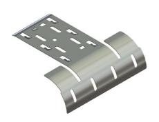
The Basic Dropout (BDO) smooths the transition of cabling dropping out of wire mesh tray. These dropouts snap into place without hardware and reduce the strain of cables as they exit or enter the tray. It mounts at the end of the wire basket cable tray parallel or perpendicular to the tray bottom.
