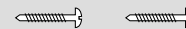
Two (2) No. 8 1½ in. (38 mm) round-head screws to securely attach the fan heater mounting bracket.
