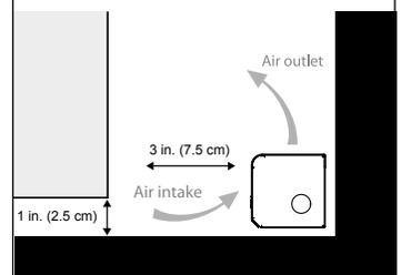
Between the front of the unit and objects located directly on the floor.
