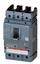
circuit breaker 3VA6 UL frame 150 breaking capacity class L 150kA @ 480V 3-pole, line protection ETU320, LI, In=150A overload protection Ir=60A...150A short-circuit protection Ii=1.5...10 x In without connection
