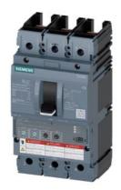
circuit breaker 3VA6 UL frame 150 breaking capacity class C 100kA @ 480V 3-pole, line protection ETU350, LSI, In=150A overload protection Ir=60A...150A short-circuit protection Isd=1.5...10 x Ir, Ii=10 x In without connection
