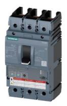
circuit breaker 3VA6 UL frame 150 breaking capacity class M 35kA @ 480V 3-pole, line protection ETU320, LI, In=100A overload protection Ir=40A...100A short-circuit protection Ii=1.5...12 x In without connection
